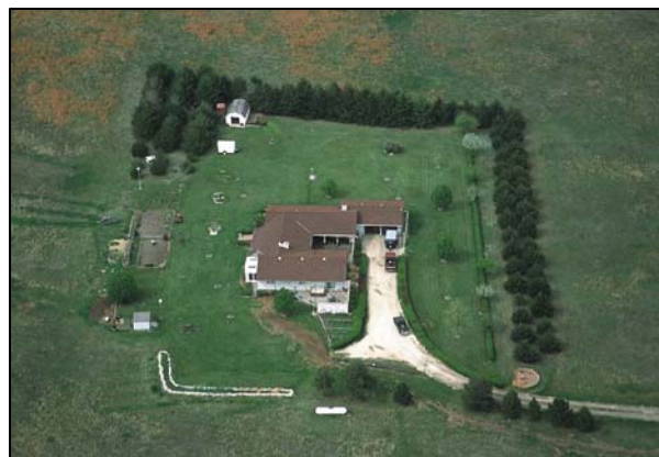
A windbreak saves energy and adds comfort and livability to homes in open country.
